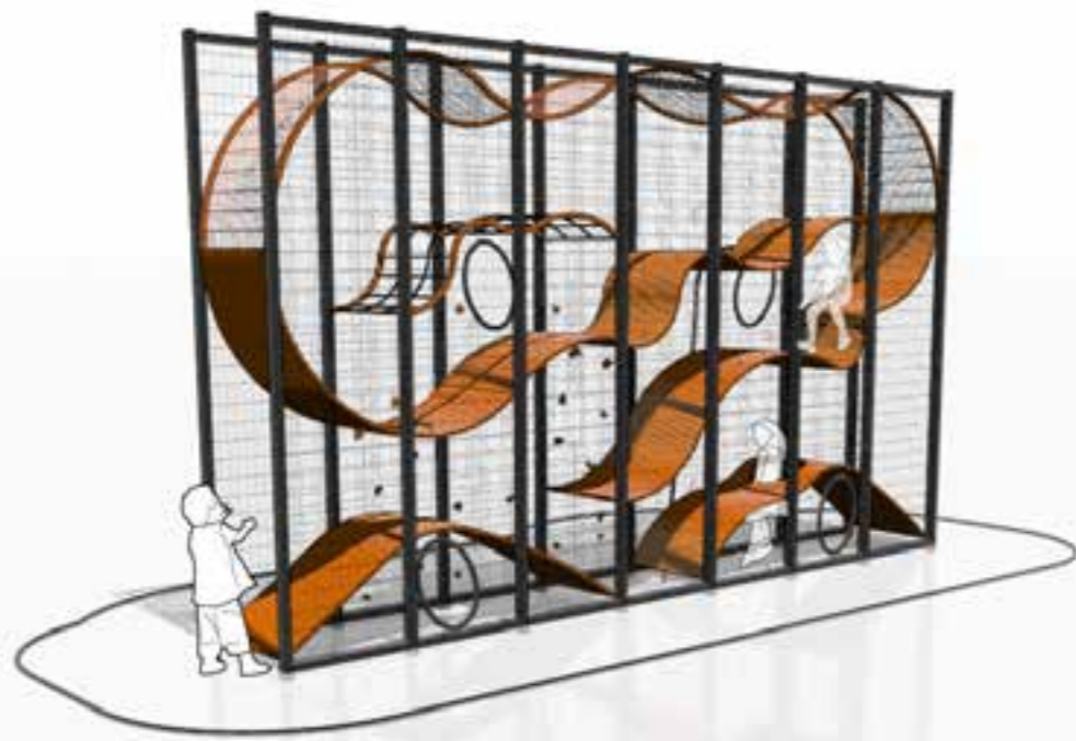
7 modules: approx. 8,3 metres long. Safety area: 11 080 x 5 180 (52,4 m 2 ) Capacity: 21 persons
